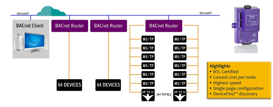
With BBMD the FieldServer BACnet Router can move data from the RS-485 trunk through firewalls and different subnets to the BACnet Client The FieldServer BACnet Router can have up to 32 devices per RS-485 port. With two RS-485 ports 64 devices can be connected without the use of a line driver
