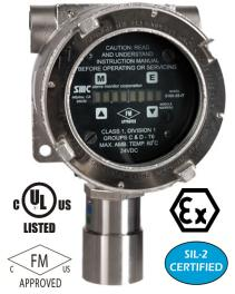
The 5100-28-IT can be used as a 4-20 mA component or as a Modbus RTU node. For higher level system capability the module can interface directly to Sierra Monitor's Sentry Controller. As part of a Sentry system the user gains capability of system Modbus serial communications, extensive diagnostic features, area and zone alarm management, WebServer interface and multiplexing sensor connections.
