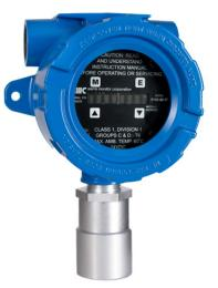
The 5100-88-IT can be used as a 4-20 mA component or as a Modbus RTU node. For higher level system capability the module can interface directly to Sierra Monitor's Sentry Controller. As part of a Sentry system the user gains capability of system Modbus serial communications, extensive diagnostic features, area and zone alarm management, WebServer interface and multiplexing sensor connections.
